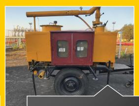
Spare hose boxes and inline inductors were attached on trailer foam tanks (one on each tank) with the help of mechanical department.
